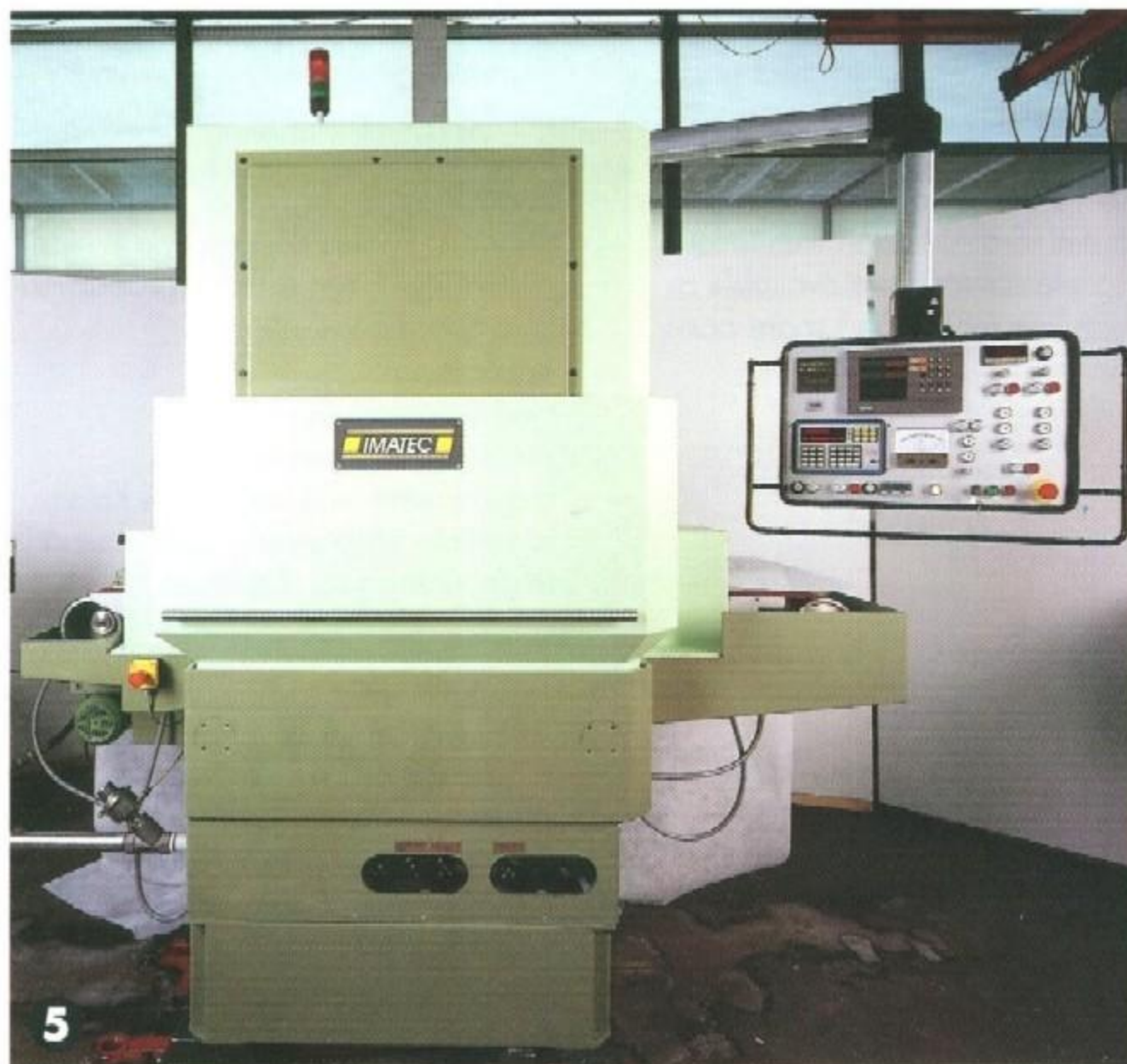
5 Machine, protection hood closed, without work piece return conveyor system.
